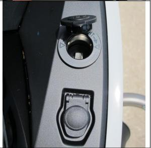
For connection to the accessory power socket, connect the supplied harness to the lighter socket (red = + / brown = -). Remove the Hirschmann connector from the existing accessory power socket and connect that lead to the mating plug on the "Y" harness at right. Connect the other mating "Y" harness plug to the accessory power socket. With this connection, the lighter socket should shut-off 50 seconds after ignition-OFF.
