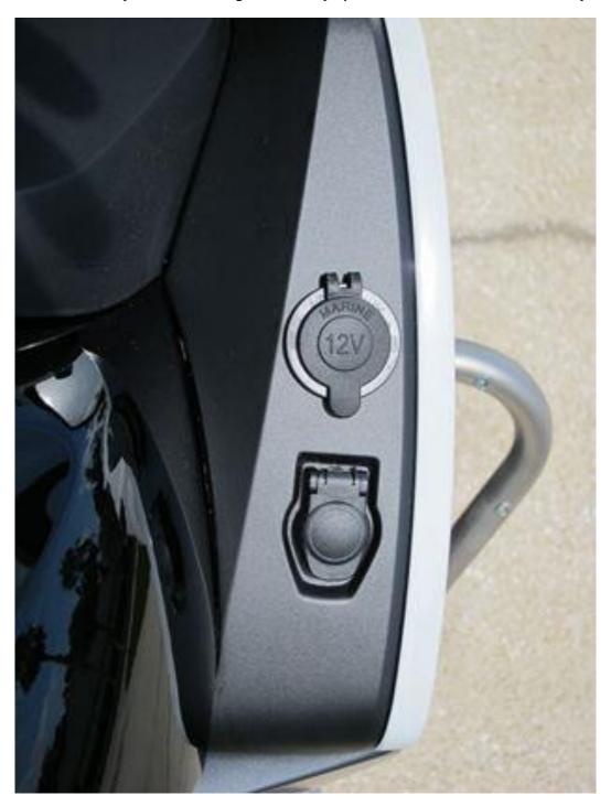
Remove RH fairing side panel (see details below). Loosen RH front protection bar to enable safe removal of the side panel without causing damage. (panel removal instructions are below if needed)
