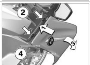
Be very careful not to damage the tabs when removing and installing RH panel.
