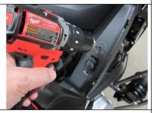
Install lighter socket through hole, install nut behind and tighten, correcting plug and weatherproof cover alignment as desired.
